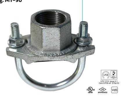
The MT-90 mechanical tee serves the same function as the MT-1 and MT-8, but uses a steel electro-plated u-bolt to save space for easier installation in tight places. The MT-90 is ideal for direct connections with sprinkler heads and drop nipples.
